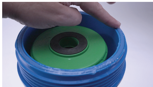
14) Use a finger to evenly spread the silicone lubricant around the O-ring. Repeat with each cartridge casing.
