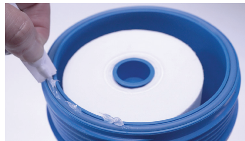
13) Apply silicone lubricant to the O-ring at the top of the cartridge casing. 1 lubricant is provided per cartridge. Repeat with each cartridge casing.
