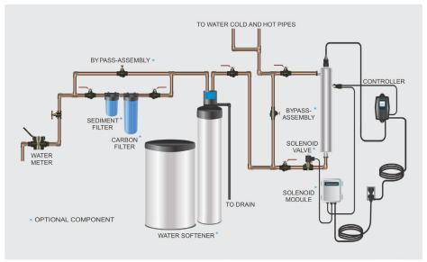
Figure 1. Recommended POE Installation Location
